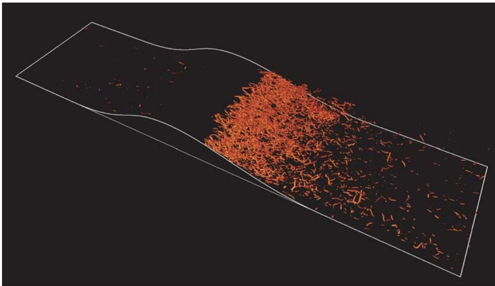
Fig. 1. Positive iso-contours of the  $Q$ -criterion ( $Q = \|\Omega\|^2 - \|S\|^2$ , where  $\Omega$  and  $S$  are respectively the vorticity tensor and the strain rate tensor) in the detection of coherent vortices on the lower wall of the simulation. Intense vortices are generated near the summit of the profile near the separation region of the turbulent boundary layer. The separation mechanisms will be investigated with respect to turbulent statistics.
