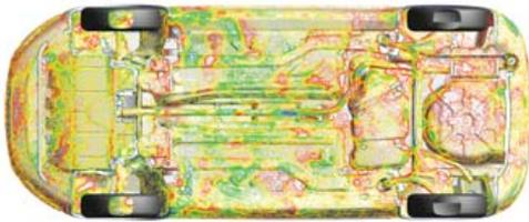
Fig. 2. Instantaneous acoustic pressure distribution on the underbody of the vehicle. The image depicts the computed acoustic pressure at a certain point in time on the surface of the vehicle underbody. In the red regions, the instantaneous fluctuating pressure is higher, while in the blue regions it is lower. This pressure distribution stimulates the underbody panels that generate noise within the cabin.
