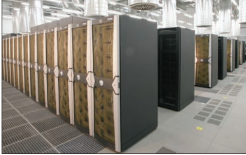
The upgraded Altix 4700 at LRZ with a LINPACK performance of 56.5 TFlop/s and a memory of nearly 40 TBytes.
