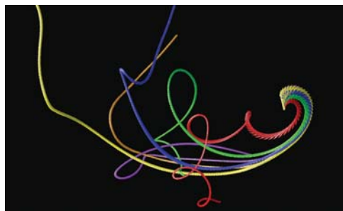
Fig. 1. Trajectories of particles with different inertia, released from the same spatial position. The red curve is a particle with no inertia (fluid element, hence following the fluid material line); the yellow curve is a particle with the largest inertia in our simulation. As mass grows, particles are less and less sensitive to small scale vorticity and to rapid velocity variations; particles with high inertia are expelled from high vorticity regions.
