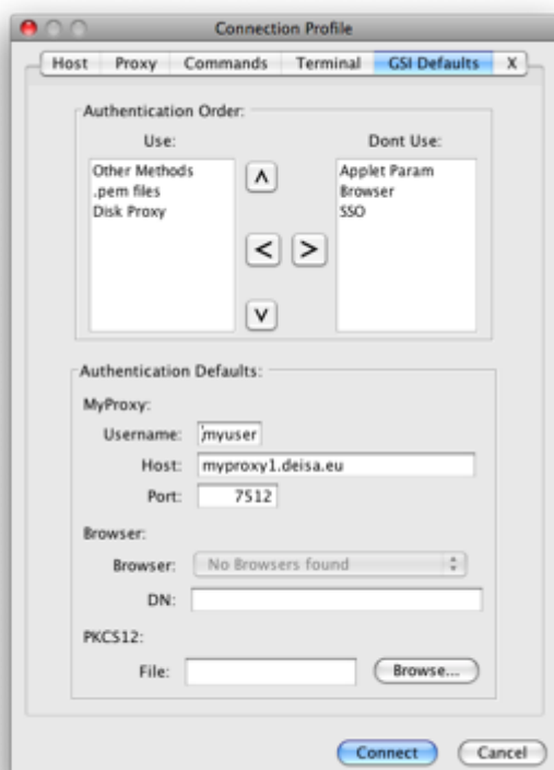
Figure 7: GSI-SSH Java Web Start application: The connection properties can be configured by clicking the "Advanced" button in the "New Connection" dialogue. In this tab, one can use the "MyProxy" method from the "Other Methods" list to fetch a proxy.
